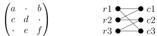
FIGURE 1. The subset of known entries of the matrix to the left correspond to the graph on the right. If a, b, c, d, e, f are sufficiently generic, then the partial matrix can be completed to rank two, but not rank one.
